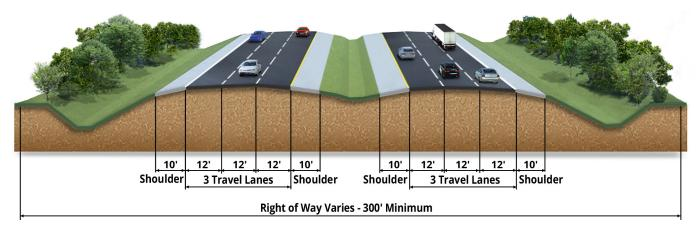
The proposed project will widen I-295 by one lane in each direction to the inside of the center lanes, increasing the existing four-lane typical section to six lanes. The project aims to improve traffic operations, enhance safety, and address congestion along an approximately 6.1-mile section from south of Heckscher Drive (SR 105) to north of Pulaski Road.
